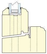
External beading can be ventilated in a flat or angled rebate. The compressed gasket is fitted in the frame grooving.
