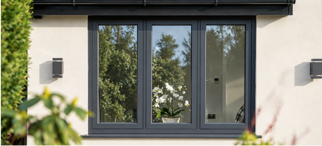
Figure A. A standard uPVC casement in a grey foil finish. This one has the flush-sash option, where the opening parts sit level with the frame. Standard sashes have an ovolo (rounded) or chamfered (angled) edge.
